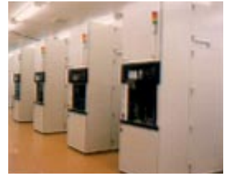
Tokyo Electron Oregon manufactures the advanced ALPHA (x)-8S series of oxidation/diffusion furnaces and LP-CVD systems.
