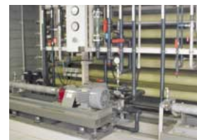
Reverse osmosis system for recovering water
